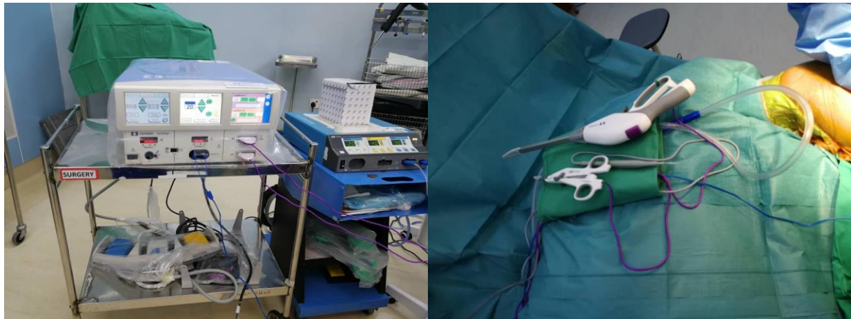
Figure 5: a) Ligasure™ console system controls b) Small and large jawed Ligasure™ handheld diathermy clippers.
