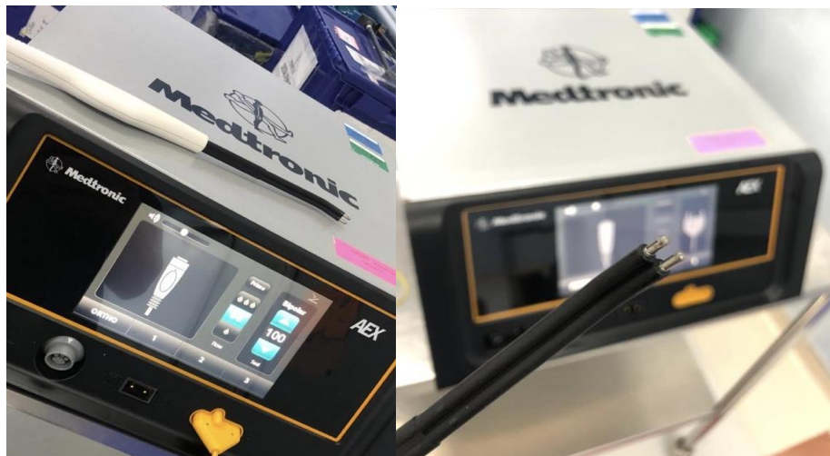
Figure 4: a) Medtronic Aquamantys™ console controls with probe. b) Aquamantys™ dual tip end probe with irrigating system
